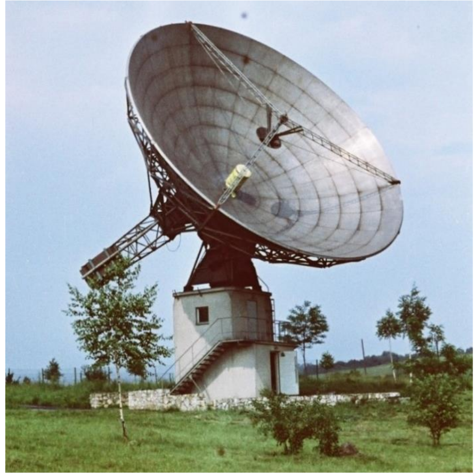
The 15-m dish with its Cassegrain focus
