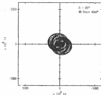
Figure 1.14 U-V Plane Coverage for QUASAT Plane
