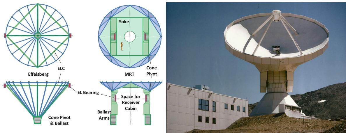
Slide 13. Homology design of the MRT compared to the original Effelsberg solution.
