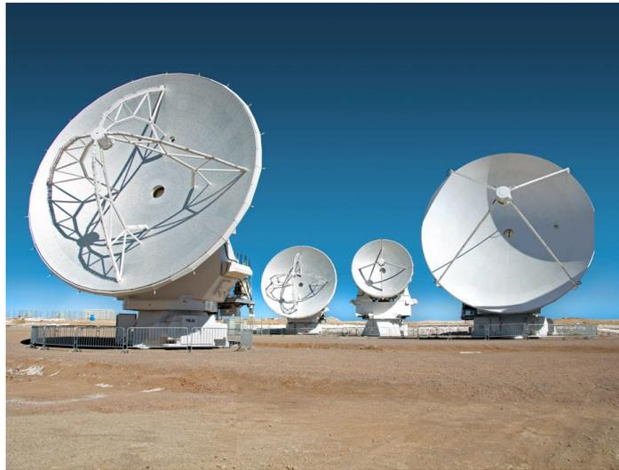
Slide 15 Pictures of ALMA antennas on Chajnantor, Chile. Foreground: the 12 m diameter antennas from “North America” (left) and “Europe” (right) , 25 of each. Background: Japanese contribution of 12 m antenna (left, 4 off) and the “compact array” of 12 dishes of 7 m diameter.
