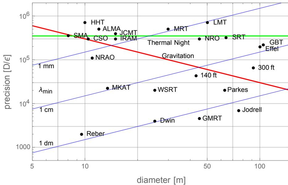
Slide 18. Radio telescopes on a "precision vs diameter" plot with von Hoerner's "natural limits" gravity and thermal; blue lines indicate "minimum wavelength".
