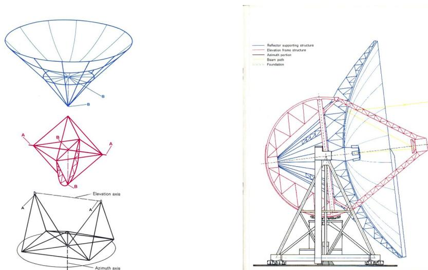
Slide 11. The design of the Effelsberg 100-m telescope.
