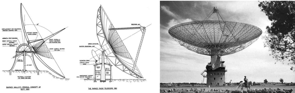
Slide 6. Parkes 64-m telescope in Australia. Original first proposal sketch (left), final design drawing (center) and the completed telescope in 1961.
