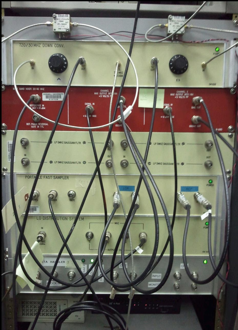
The portable fast sampler
