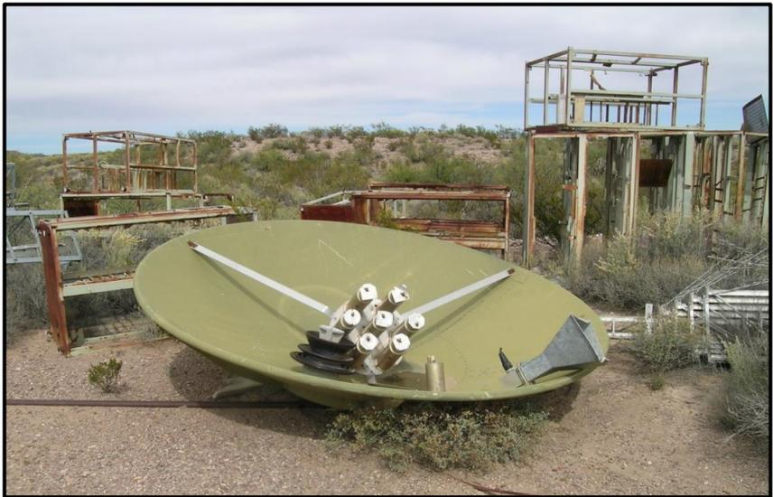
**The 2<sup>nd</sup> SNORT antenna with its prime focus no longer in an optimally located position.**
