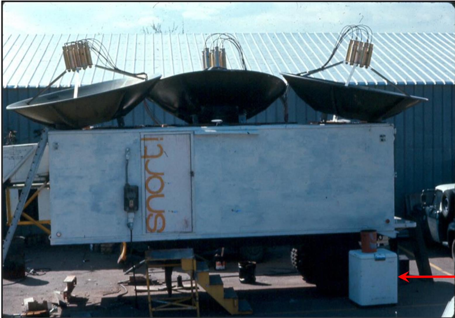
**Close-up picture of the SNORT trailer and its 3 telescopes, each with 7 feeds, which yielded 21 separate beams on the sky searching for a microwave pulse from an exploding star.**
