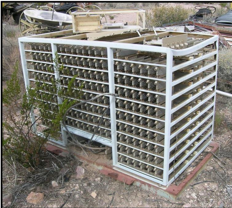
**The Beamformer rack full of 12 and 16-way splitters (lower left).**
