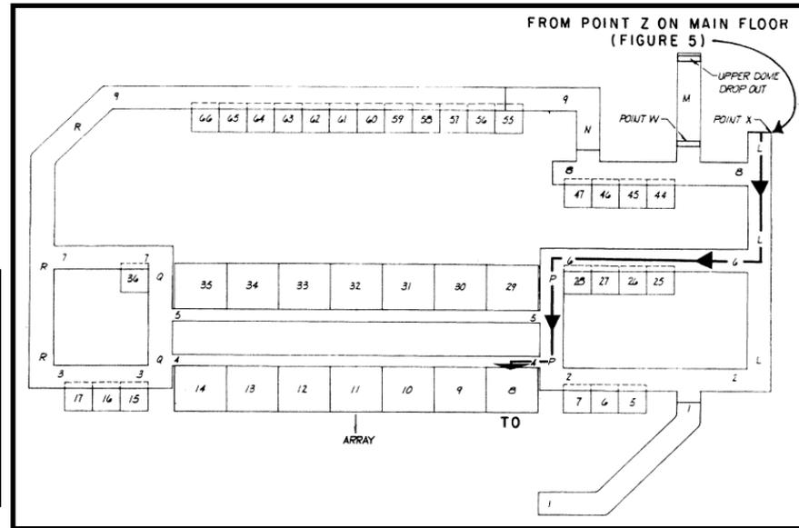
*“Street map”* of the numerous electronic racks on the Receiver Dome Main Floor of the MAR-I
