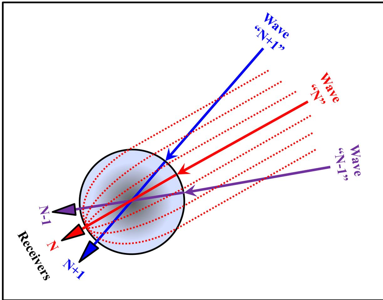
Thus it is possible for multiple signals to be received simply by placing more receivers on the sphere's periphery.
