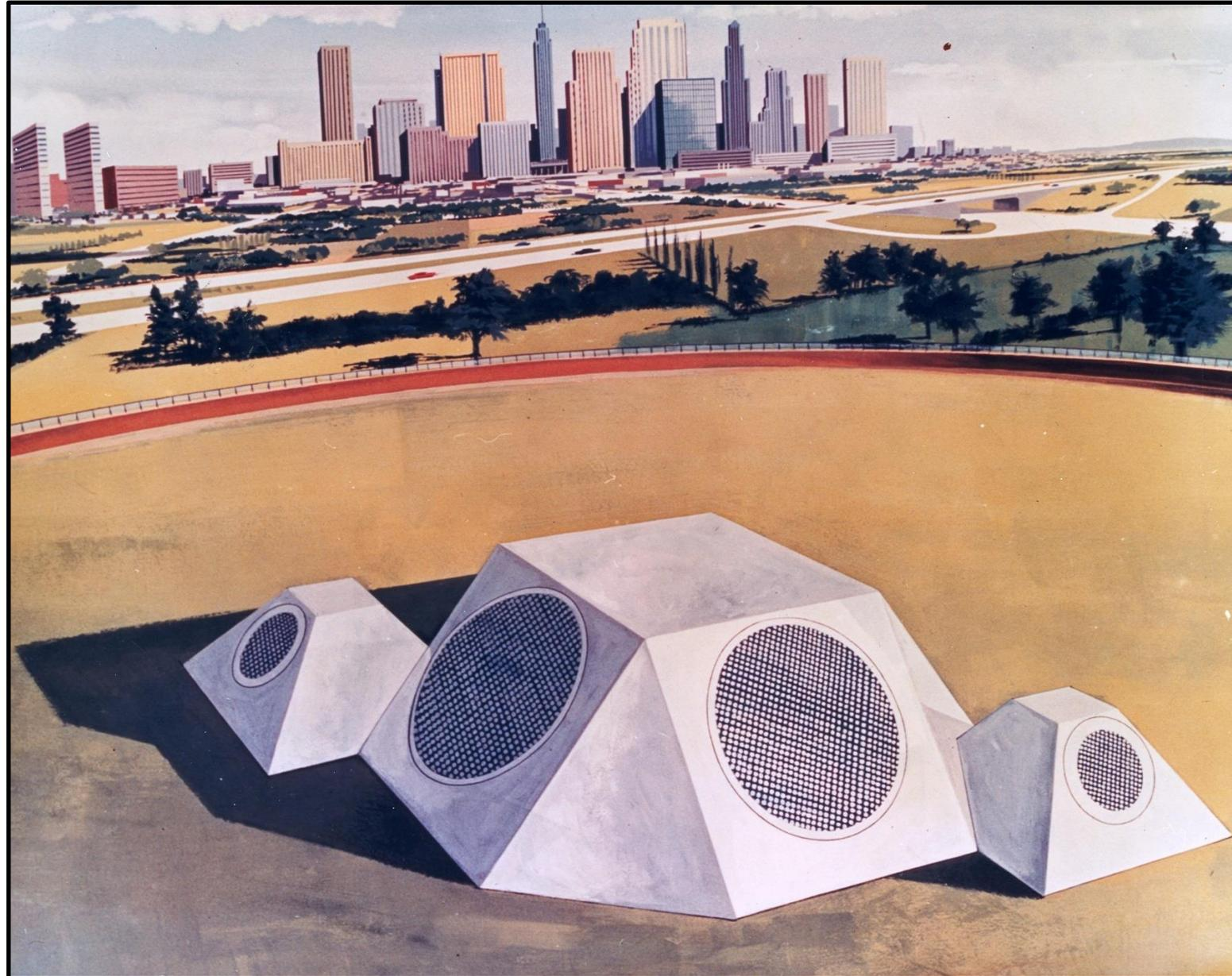
**Gone were the domes of the MAR-I, being replaced by a large 8-sided structure for the receiver arrays, with smaller truncated pyramids for the transmitter arrays.**
