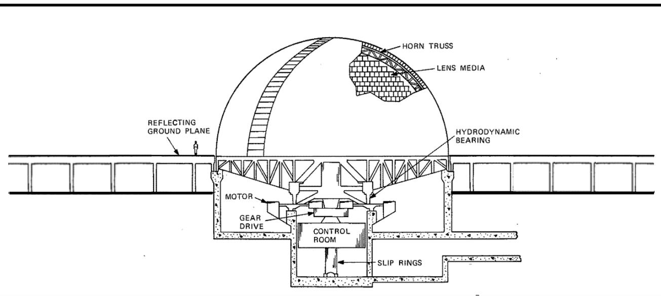
Cutaway view of the ZAR Rx antenna built showing the reflecting ground plane, and one of the three horn trusses.
