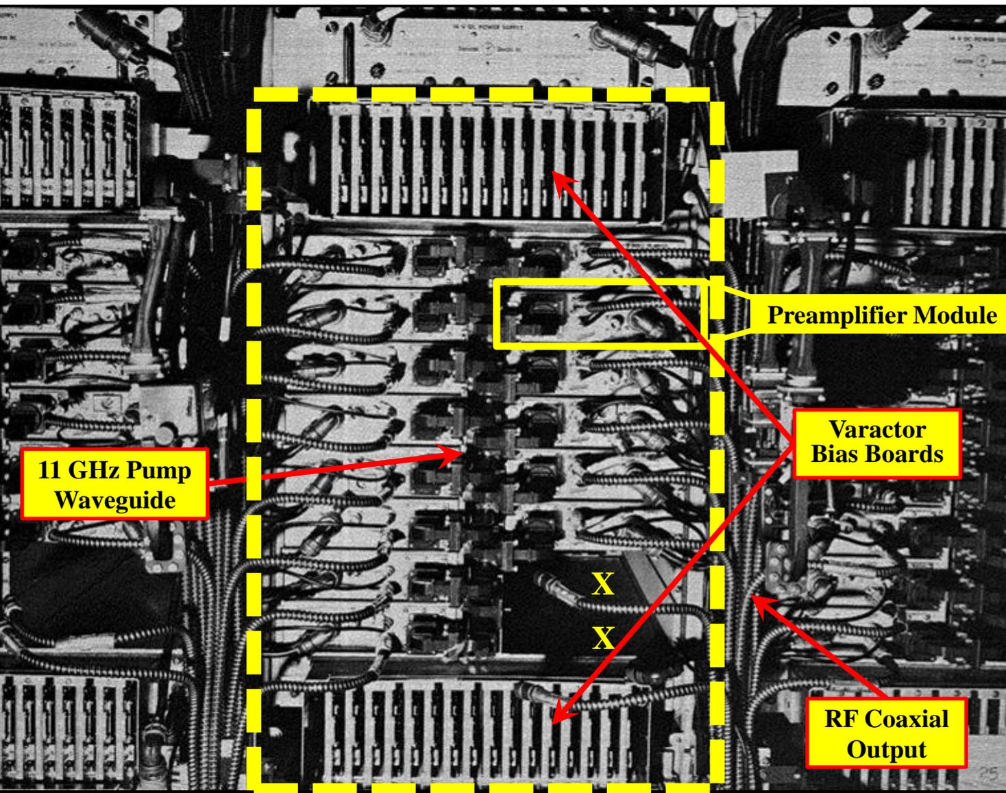
The signal received by each of the *Antenna Elements* first passed through a Western Electric *Preamplifier* unit.
