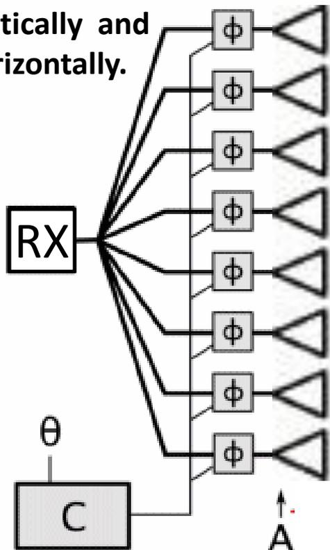
The more elements, the wider the aperture, and the narrower the beam.
