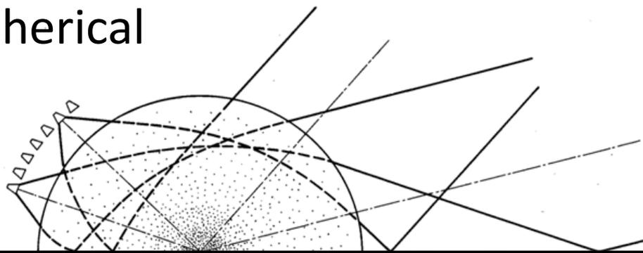
Incoming signals are reflected by the ground plane & focused by the dielectric lens to horns on the opposite side of the lens.
