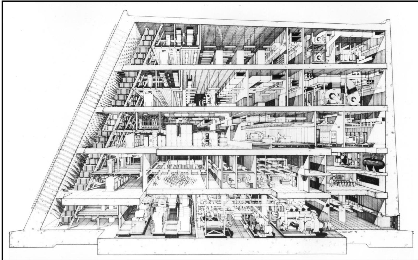
The reinforced walls were 4 to 7 feet thick.
