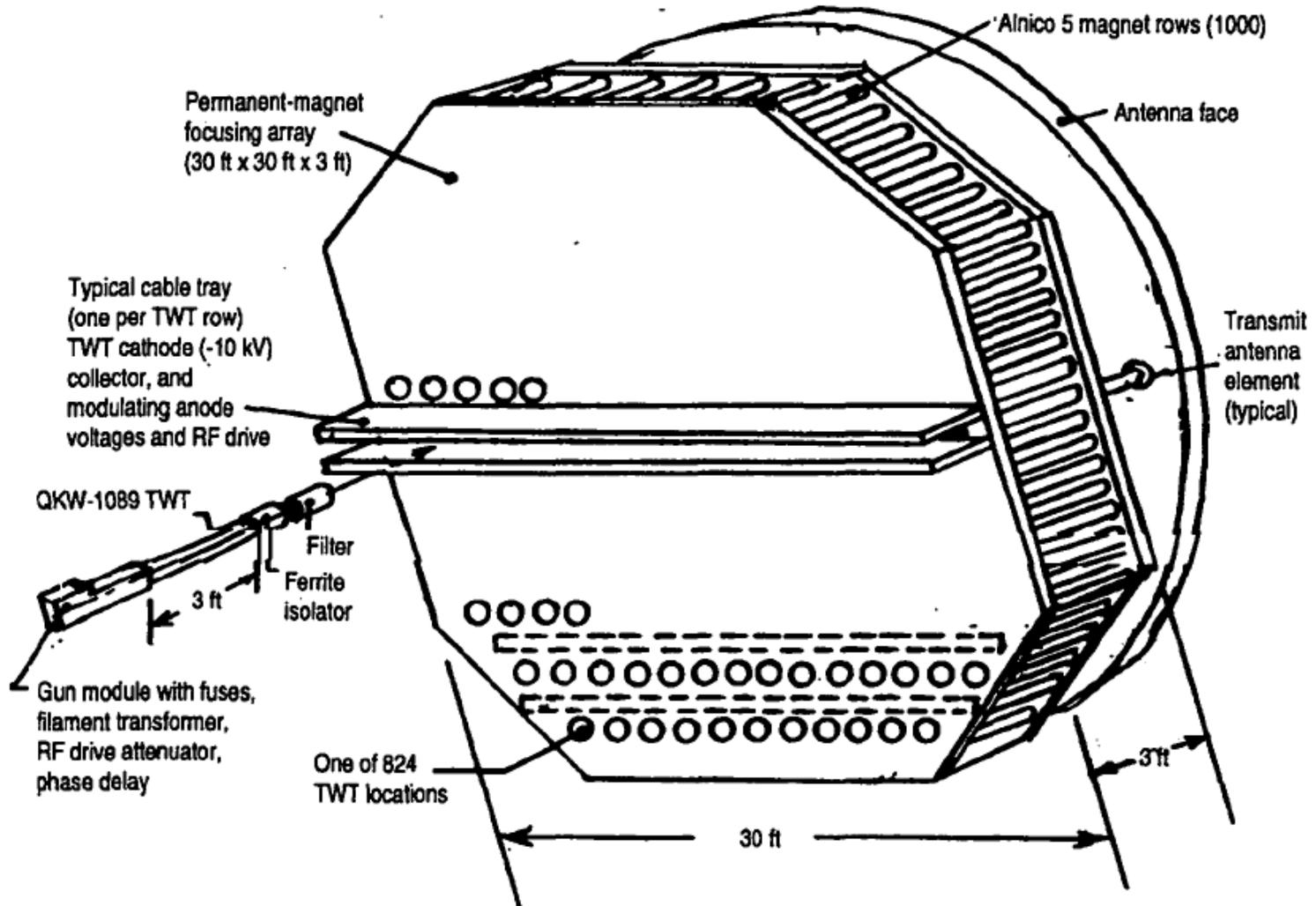
Figure 11-17. Simplified representation of the MAR-I transmitter-array face.
