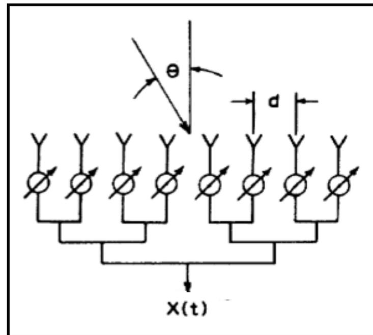
In a *Corporate-Fed Array*, like the MAR-I, the transmission lines connecting the elements to the beamformer are all of equal length.
