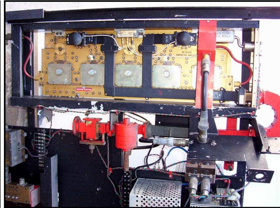
View of the IAR receiver showing the gold stripline paramp that had been removed from the MAR-I Preamplifier Module donated by Stirling Colgate.
